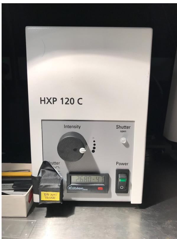
Figure 1: The image above shows the power box for the lamp and shutter.
