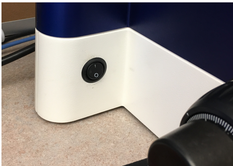
Figure 2: The image above shows the location of the power switch for the microscope.
