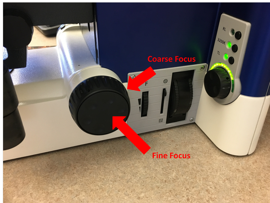
Figure 6: The image above shows the focus adjustment knob. The outer element of the knob adjusts the coarse focus, while the inner element adjusts the fine focus.
