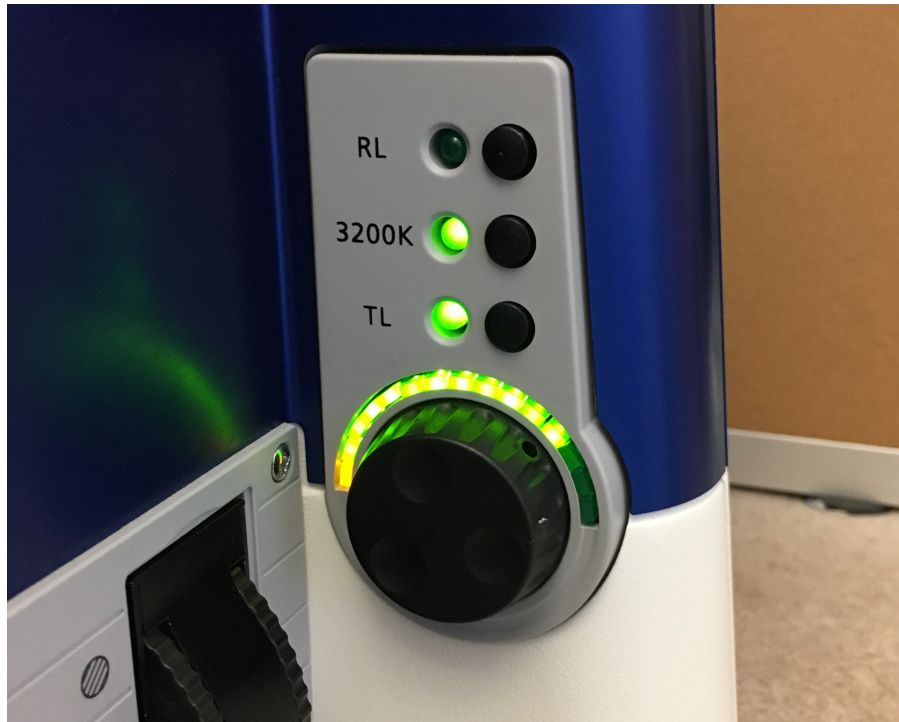
Figure 3: The image above shows the location of the 3200K illumination button.
