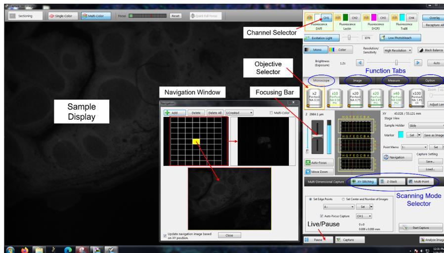
Figure 4: Overview of Focusing and Navigating the sample.
