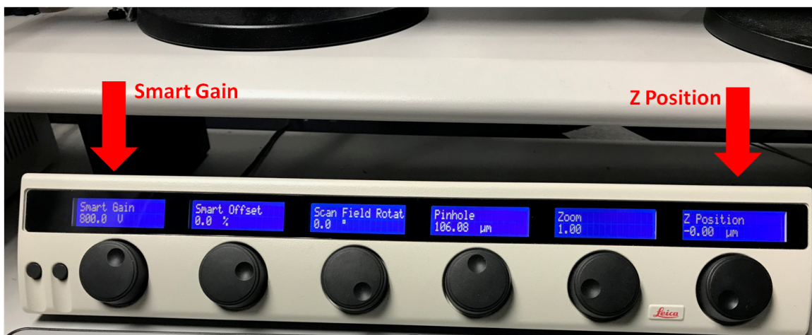
Figure 8: The image above shows the smart board where the Smart Gain and Z- Position knobs are located.
