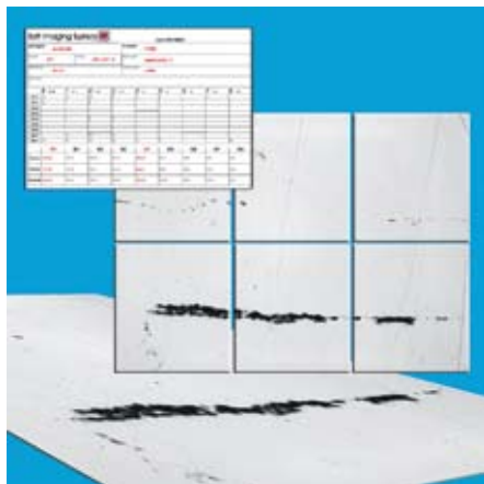
Fig. 21: The analysis of non-metallic inclusions according to DIN, ASTM and JIS requires the processing of areas up to 1000 mm 2 while the sulphide and oxide inclusions to be analysed are themselves less than micrometres wide. No camera is available offering such a large CCD sensor. The image processing solution stitches single overlapped images to give one high resolution image together.
