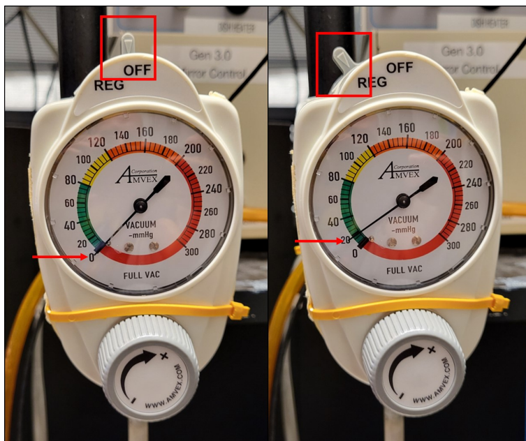
Figure 8: The regulator should register a pressure when turned on.
