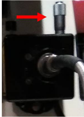
Figure 6: Knob to adjust the position of TIRF excitation light a rear focus of objective.
